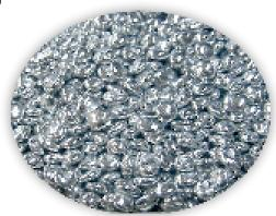
Lab Armor Beads keep lab water baths dry and protected from water-borne microbial contaminants.
