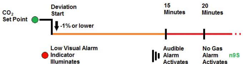
Low and No Gas Alarms Timeline
