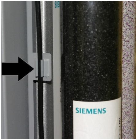
Figure 7: Water Output Line Secured
